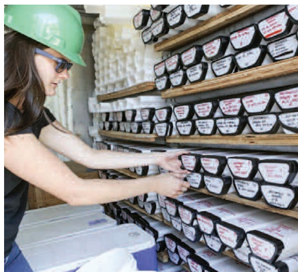
Checking core samples from the ocean floor on a research vessel (Photo: N.S. Department of Natural Resources and Renewables)
